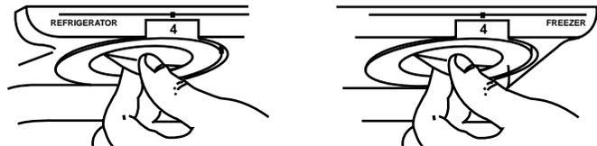
**NOTE:** To turn your refrigerator off, turn the refrigerator control to the word OFF or until the word OFF appears, as shown below. Your product will not cool when the refrigerator control is set to OFF.
