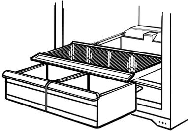
3. Replace the cover by fitting the cover tabs into lowest cabinet slots and pushing them in. Lower the front retainers into place.
