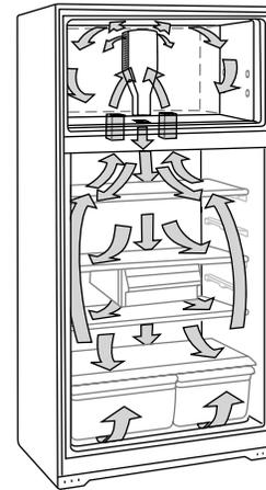
**Do not block any of these vents** with food packages. If the vents are blocked, airflow will be prevented and temperature and moisture problems may occur.
